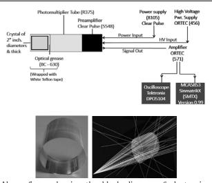
Above figure showing the block diagram of electronics used in the experiment. Below is the actual plastic scintillator photo.
