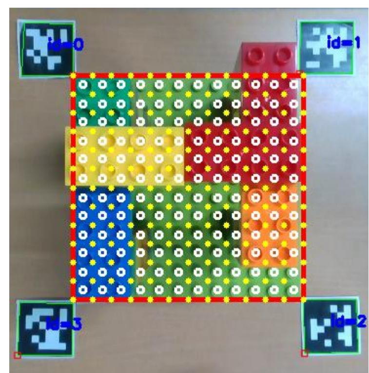
ArUco markers are used to define the grid space for assembly. Camera calibration is still required to test integration with OpenGL + ROS2.
